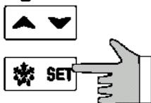
Press the SET key for more than 2 seconds to change the Set point value. The value of the set point will be displayed and the ❄ LED starts blinking. To change the Set value, pushing the ▲ or ▼ arrows within 10 sec. To memorize the new set point value, pressing the SET keys again or wait 15 sec.
