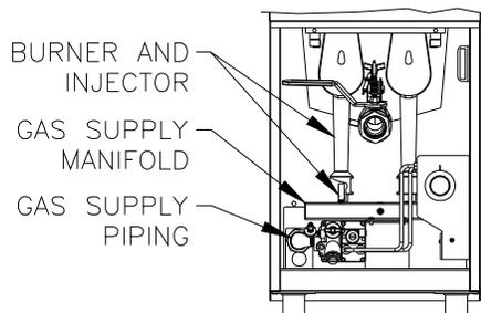
ADJUST GAS SUPPLY COMPONENTS IF NECESSARY. ENSURE THAT THE INJECTORS ARE PERPENDICULAR TO THE MANIFOLD AND PARALLEL TO THE BURNERS.
