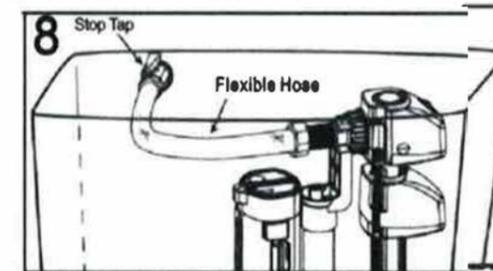
**8. IF STEP 7 IS COMPLETED, SKIP THIS STEP.** Fit off stop tap then connect rear water inlet valve to stop tap. Fill cistern and ensure correct water level.
