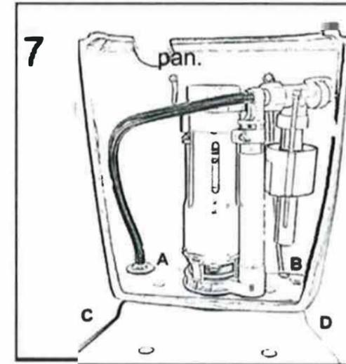
**7. IF BACK INLET, SKIP THIS STEP.** Remove cap from cistern plug A or B at base cistern. Connect flexible hose to cistern plug A or B depending on location of stop tap. Complete stop tap connection to underside of cistern plug C or D. Fill cistern and ensure correct water level.
