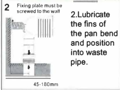
**2. Lubricate the fins of the pan bend and position into waste pipe.**
