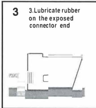
**3. Lubricate rubber on the exposed connector end**
