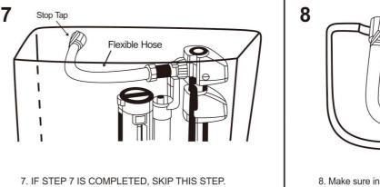
Fit off stop tap then connect rear water inlet valve to
