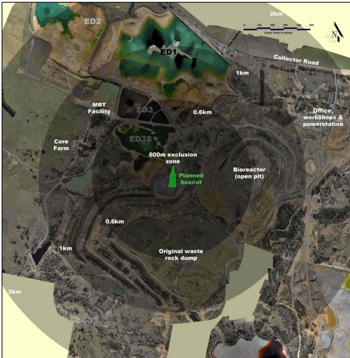
Figure 4.2 – Site layout and blast exclusion zone
