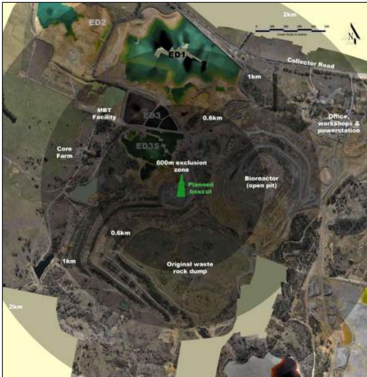
Figure 4.2 – Site layout and blast exclusion zone
