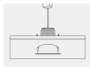
Connect driver and luminaire together. Pull back springs and load unit into ceiling.
