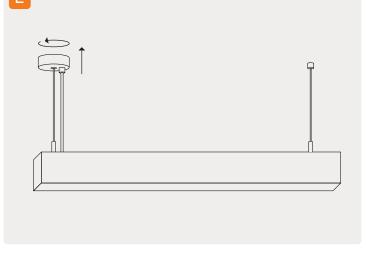
Twist the canopy clockwise to disconnect the base from the canopy. Mount the base to the surface.
