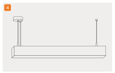
Adjust suspension height to desired length, then cut off any excess cable. Max cable length is 2m.
