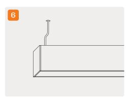
Detach and remove the suspension cables.
