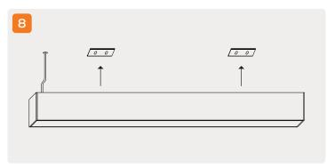
Re-attach heatsink, diffuser, and end cap by following steps 1–3 in reverse.
