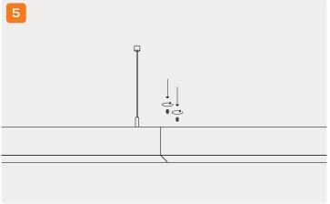
Connect adapters from both fittings. Wire suspension marked above is optional.
