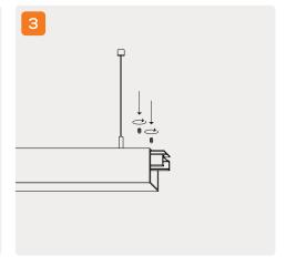
Remove screws shown in diagram. Pull off end caps, and pull out adapters.
