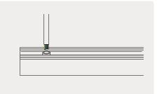
Disconnect the power cable from the fitting. Disconnect the earth connection from the fitting. Disconnect the remaining cabling to the power cable from the wiring terminal. Pull the cable through to remove from the fitting.
