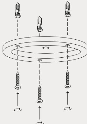
Screw mounting plate into ceiling.
