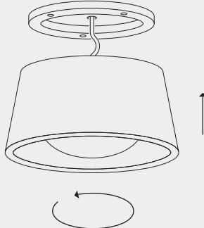
Twist counter-clockwise to connect fitting to secured mounting plate.
