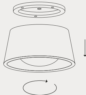
Twist clockwise to remove the mounting plate from the fitting.
