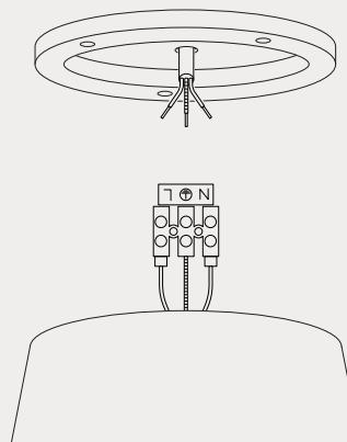
Pull power cables through mounting plate and connect power.
