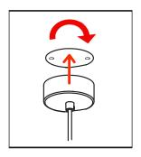
2a) Pull cable through the ceiling mount and connect to fitting cables b) Half turn twist the canopy into the base plate in the ceiling
