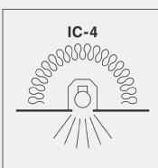
Suitable for residential or commercial use in Australia and New Zealand. Fitting may be abutted and covered according to AS/NZS 60598.2.2:2016, however for optimal efficiency we advise that the luminaire is not covered when installing.
