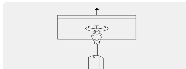
**2** Connect the driver to the mains power socket - located in the ceiling cavity. Ensure the control gear is placed above any insulation.
