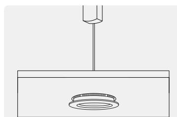
**4** Pull back springs and load unit into ceiling.
