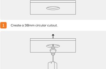
Connect the driver to the mains power socket - located in the ceiling cavity. Ensure the control gear is placed above any insulation.
