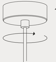
Twist the canopy into the base plate.
