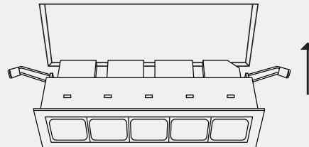
Pull back springs and fit luminaire into ceiling.
