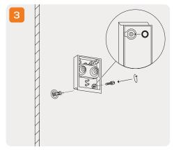
Please ensure the screw anchor & rubber ring are used when installing the back plate to retain the IP
