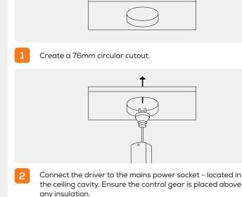
Suitable for residential or commercial use in Australia and New Zealand. Fitting may be abutted and covered according to AS/NZS 60598.2.2:2016, however for optimal efficiency we advise that the luminaire is not covered when installing.
