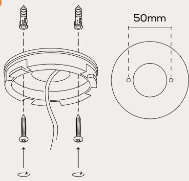
Twist base counter-clockwise to unlock.
