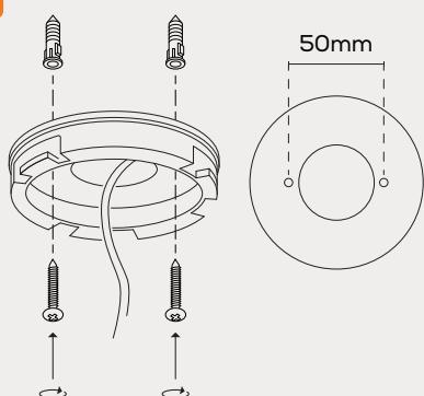
Twist base counter-clockwise to unlock.
