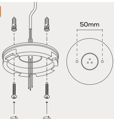
Twist base counter-clockwise to unlock.
