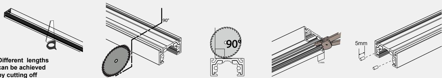
If needed, cut the linear profile to the desired length through laser cutting (recommended operation) or alternatively with a circular saw designed for metal profiles. After the cut is made, rectify and shorten the outer ends of the copper conductors inside the profile with pincers.
