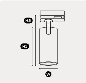
**DIMENSIONS** **H1** 125mm **W** Ø70mm
