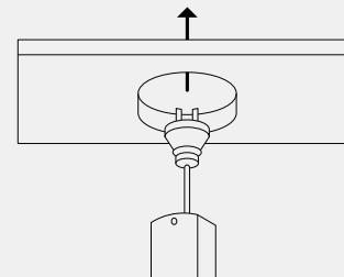
2 Connect the driver to the mains power socket - located in the ceiling cavity. Ensure the control gear is placed above any insulation.
