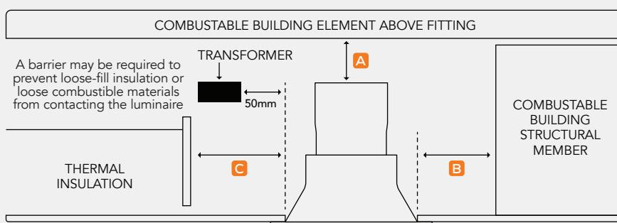
A Height Clearance To Building Element (HCB) 0mm
