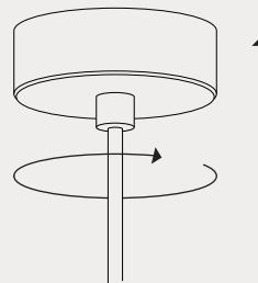
Twist the canopy into the base plate.
