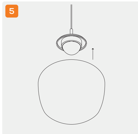
Attach glass shade to the LED head.
