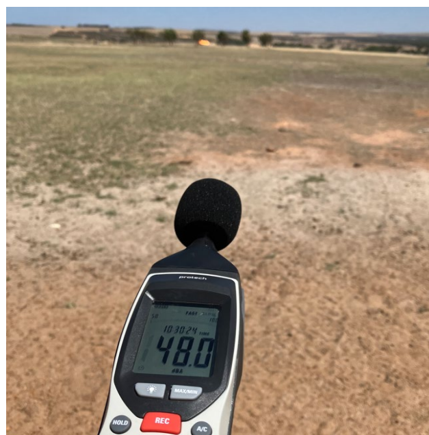
Image: Sound level meter in the foreground, with flaring operations at Waitsia 17 in the background, approximately 1.5km from the source.
