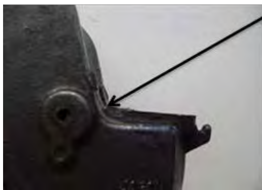
Photo 3: Steering bracket with the turning stop removed
