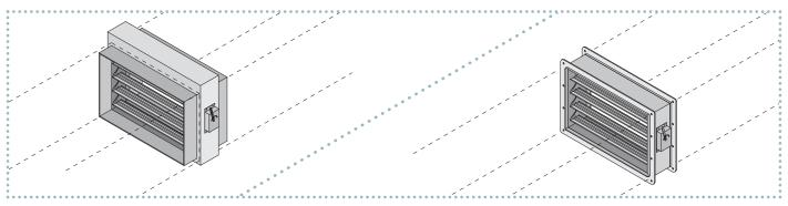
All types of damper systems can be used where appropriate, with provision for access to these items for maintenance purposes. Details on the right show installation of dampers within DURADUCT systems.
