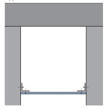
4-sided application using drop rods and cradle angle support.
