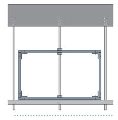
• 2-sided application using structure soffit as other two sides.
