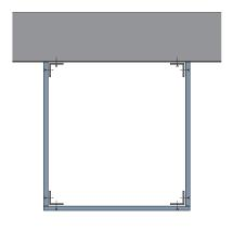
4-sided large duct, with stiffeners to ensure cross section of duct is maintained.
