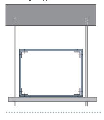
• 3-sided application using structure soffit as 4th side.
