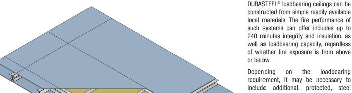
Depending on the insulation performance requirements, it may or may not be necessary to include additional cover fillets over the steel sections to retard the conduction of heat through the ceiling construction.
