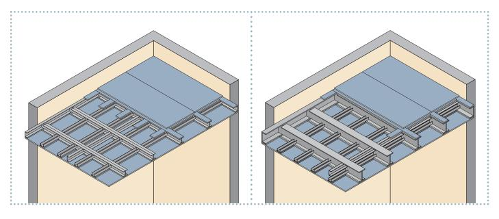
DURASTEEL® ceiling constructions can be used to create one, two or three sided enclosures. These can be used as plenums, services enclosures or to provide compartmentation.
