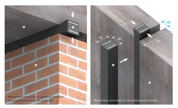
Up to -/240/240 fire resistance in accordance with the requirements of BS 476: Part 20: 1987 and/or AS 1530: Part 4: 2014, depending on applications and types of penetrating elements. Movement joints at the top of the hollow block and cavity walls AND the cavity within the hollow block walls must be sealed for a minimum one strip of PROMASEAL® FyreStrip, otherwise the hollow block and cavity walls will need to be capped
