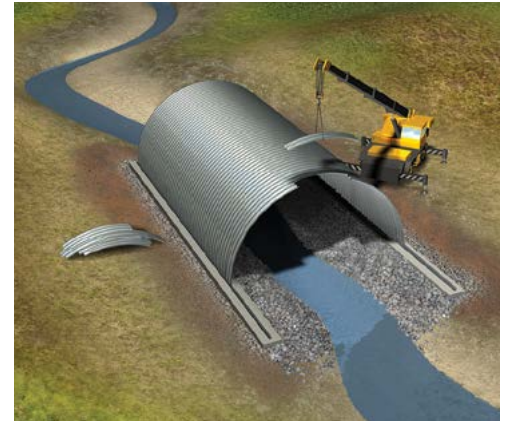
Plates then attach individually to make up other arch segments.
