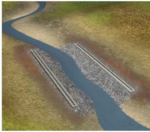
Reinforced concrete footings are cast over the prepared site.
