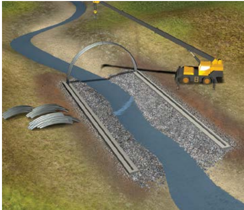
Then, it is lifted into place and bolted to the footings on either side.
