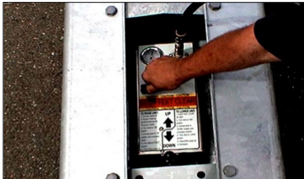
Move the selector handle from the LOCK position to the ON position
