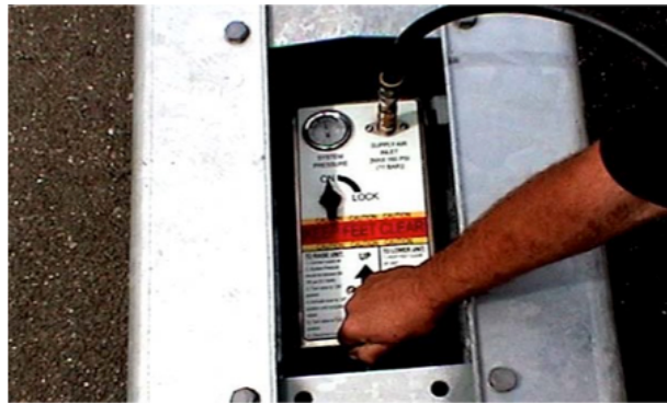
Activate the jack by moving the direction handle located on the end of the panel in the UP or DOWN position.
