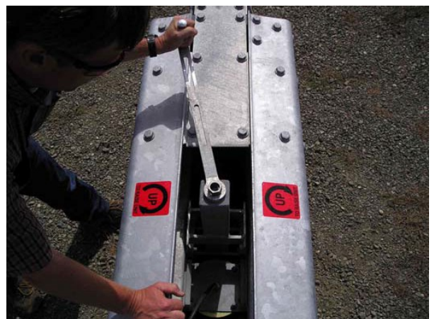
Figure 6 Manual Jack System
