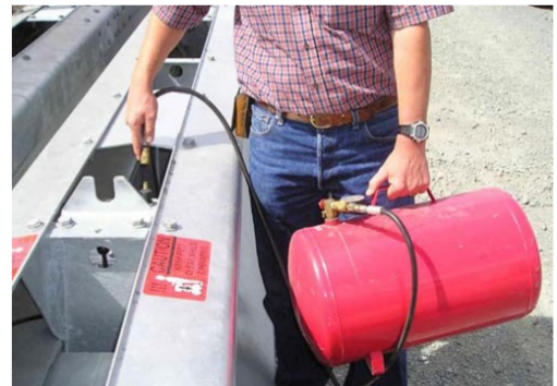
Figure 7 Air Supply Bottle for Pneumatic Raise/Lower Option
