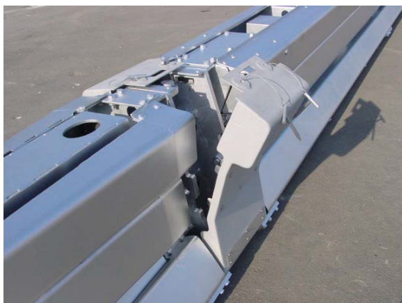
Figure 3 Rotate Cover Outward
