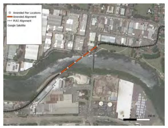
Figure 4-1: Layout of the Bridge between Camellia and Rydalmere
