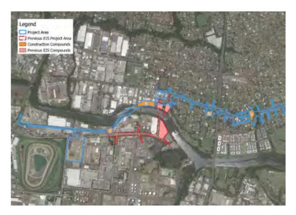
Figure 2-4 Construction compound locations – map 1
