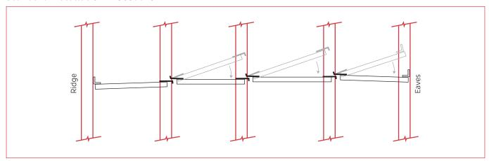
$\textbf{Note:} \ \, \text{As the eaves and ridge braces are bolted, there is a 25mm offset to the bracing line.} \ \, \text{This offset can be aligned, refer Fastbrace 2.3.8.1.}$
