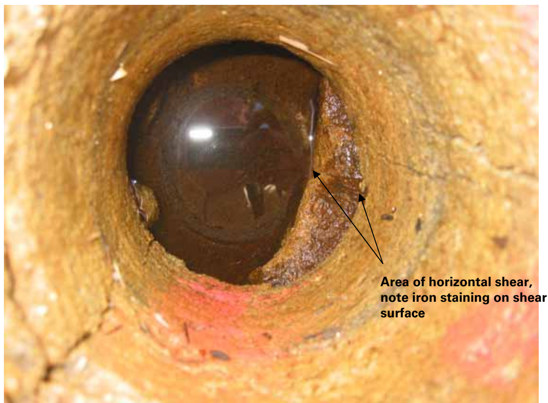
Figure 24: Incremental Subsurface Horizontal Shearing in a Vertical Borehole, Waratah Rivulet, 2007
