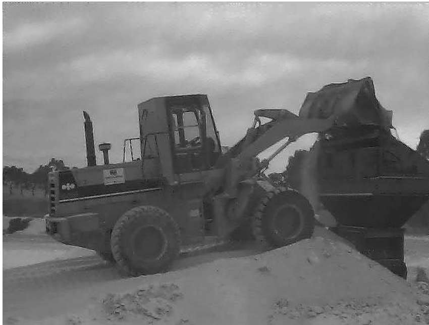
Figure 3: Komatsu WA 200 Front Loader loading into screening plant
