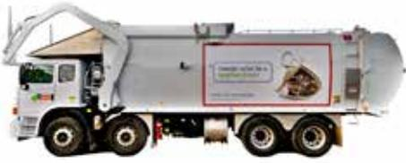
31 m<sup>3</sup> capacity. Used to collect waste. They require a 6.5 m clearance to service waste hoppers.
