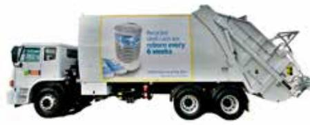
24 m<sup>3</sup> capacity. Used to collect recyclables. They require a 4.3 m clearance to service recycling hoppers.
