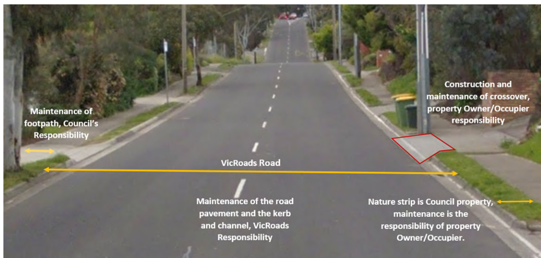
Figure 2. Operational Responsibility on Arterial Roads
