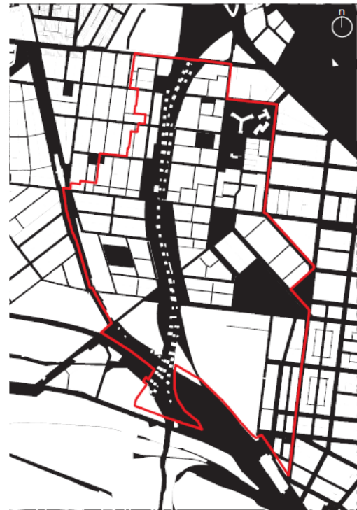
Figure 3.8: Proposed pedestrian permeability as indicated by extent of the public realm (black) - with new parks, streets and laneways shown.
