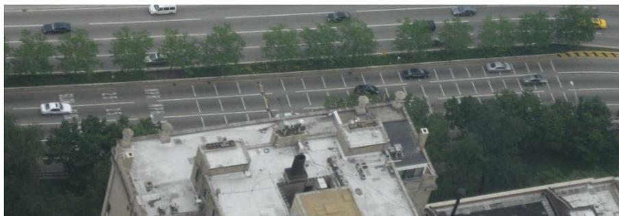
**Figure 5: Reducing speeding through spaced lines**
