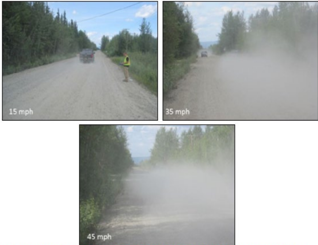
Figure 4.1. Fugitive dust created by a vehicle at different speeds (photos courtesy of Tom Moses)
