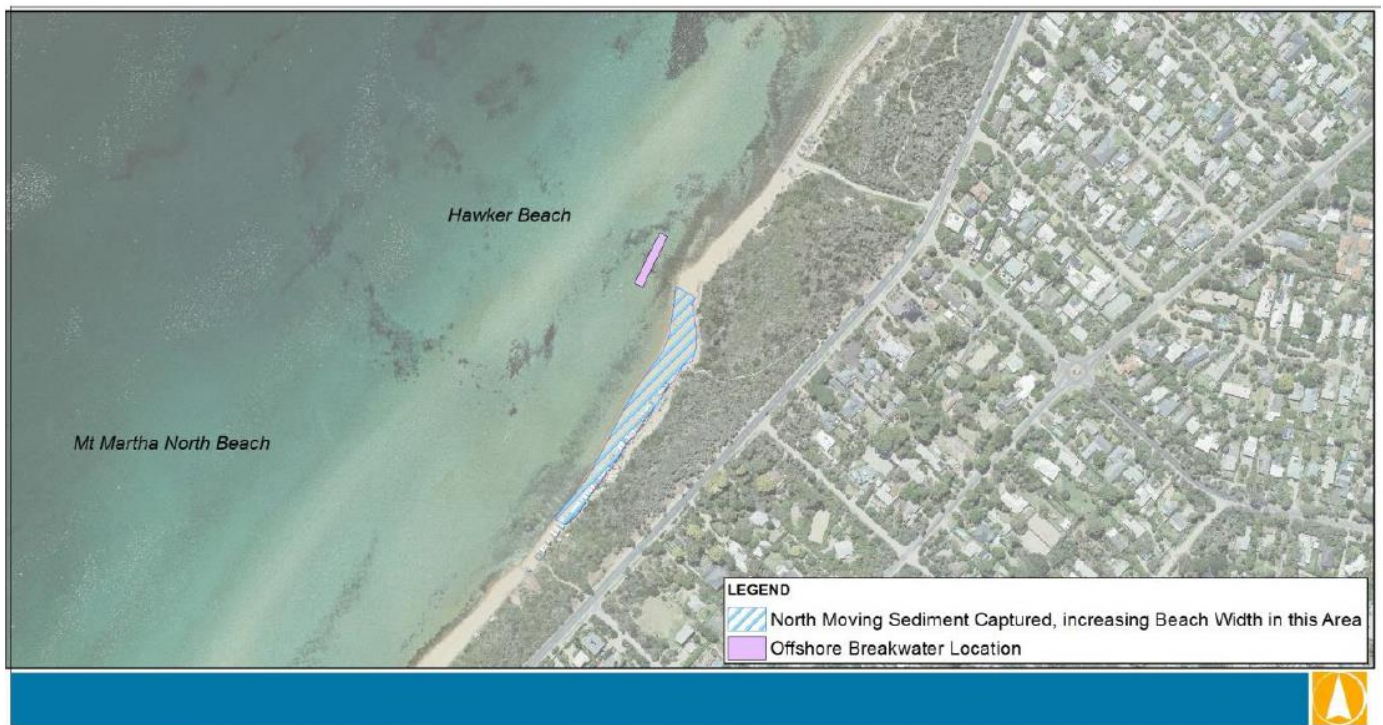
Figure 6: Illustration of small nearshore reef and renourishment, from Mount Martha North 2017 coastal processes study.
