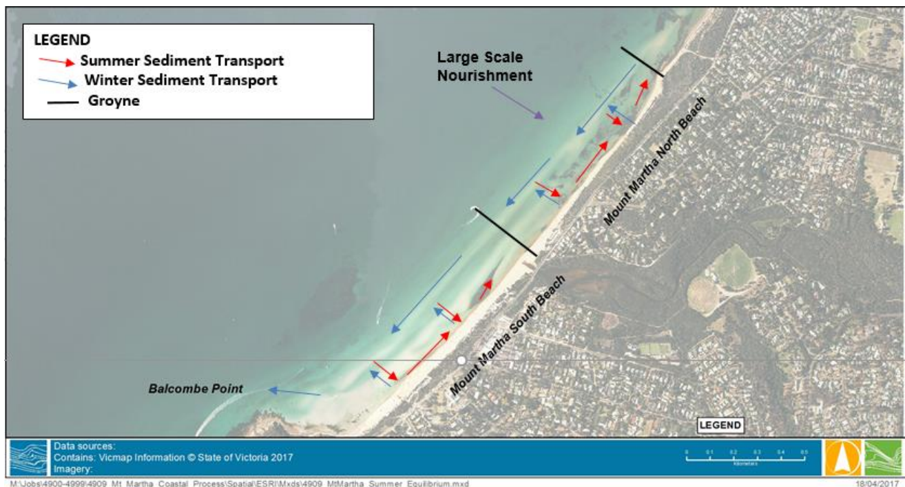
Figure 1: Illustration of large groynes and a large scale renourishment, from Mount Martha North 2017 coastal processes study.
