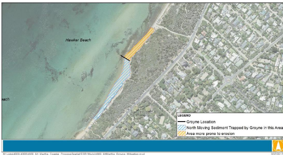
Figure 4: Illustration of sand movement resulting from installing a small groyne combined with a renourishment, from Mount Martha North 2017 coastal processes study.
