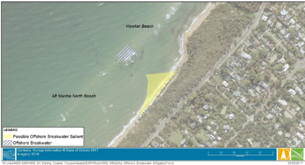
Figure 2: Illustration of large off shore reef and renourishment, from Mount Martha North 2017 coastal processes study.
