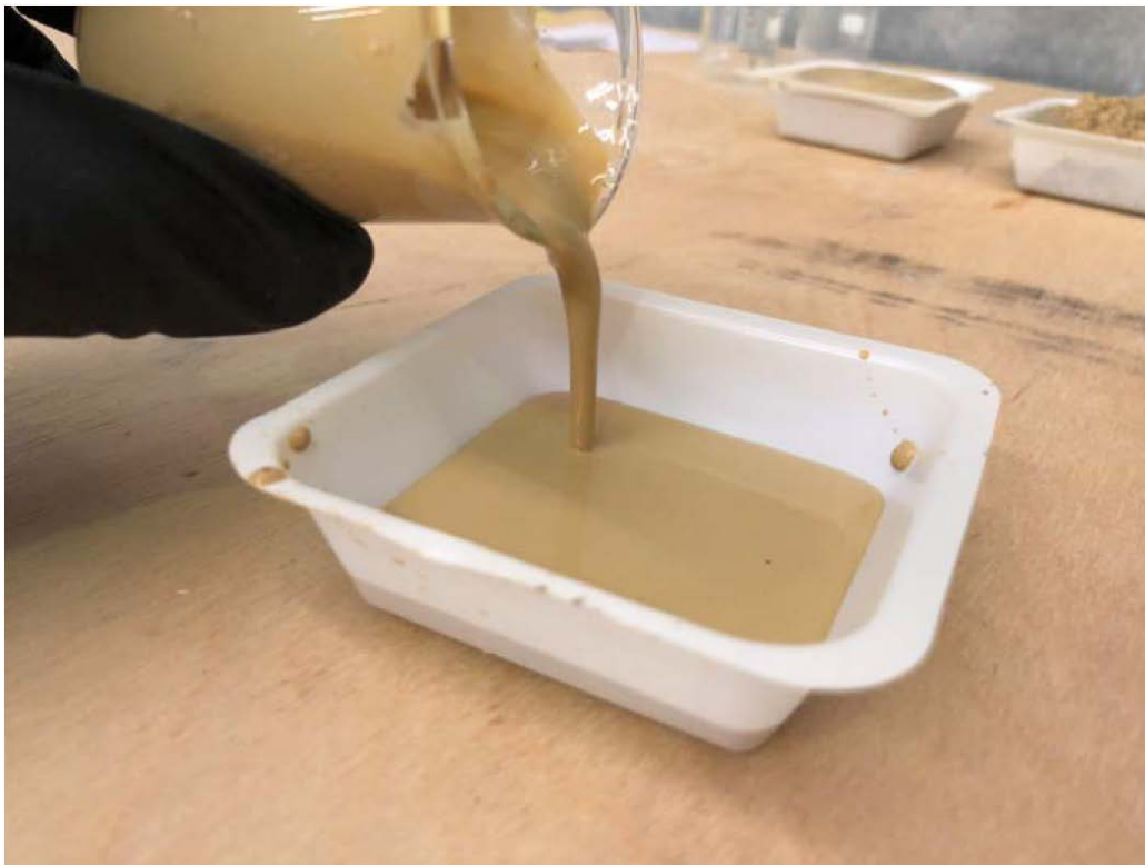
Figure 1 Fingerboards 30% solids fine tailings after thickening
