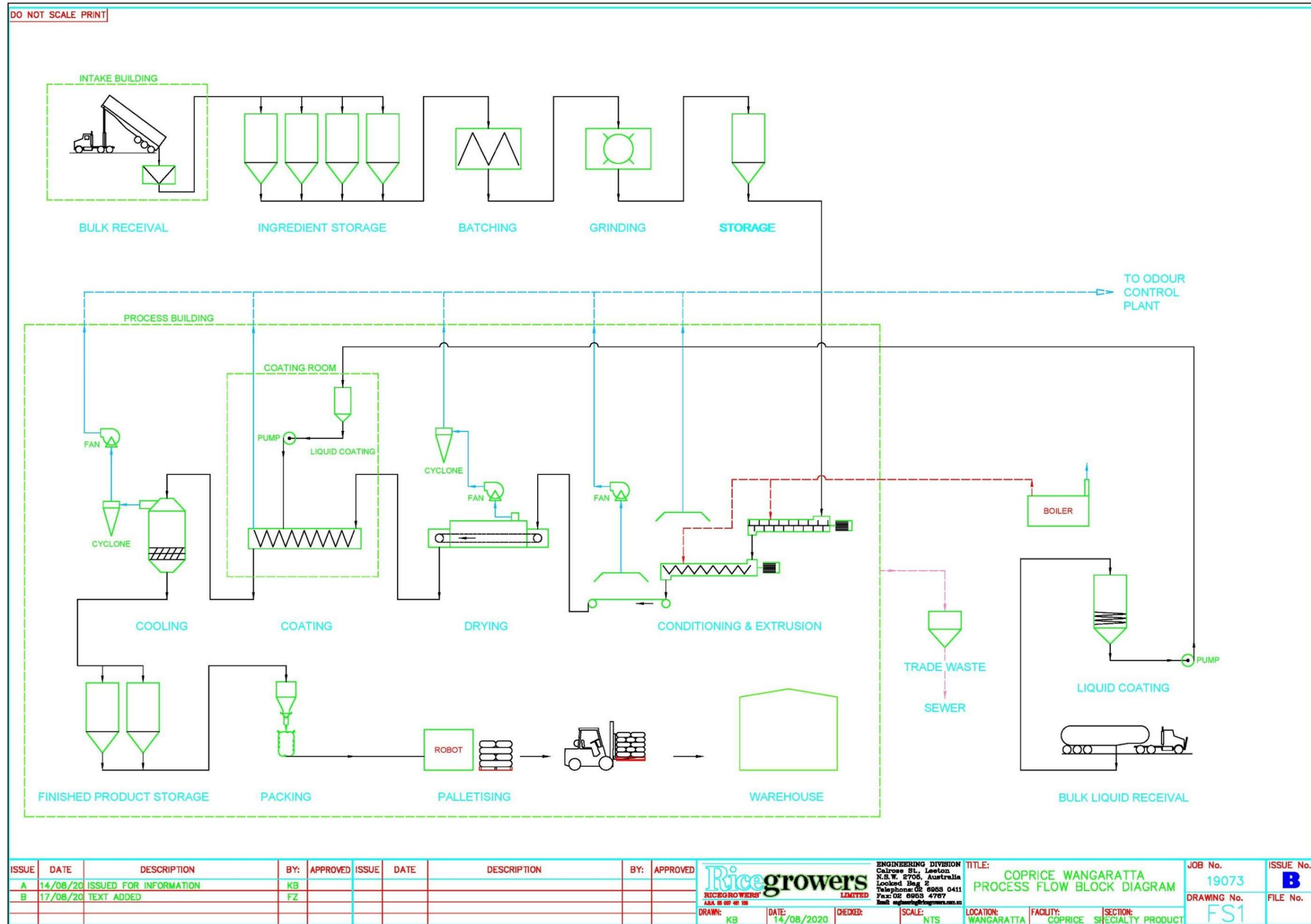
Figure 2 – A process flow diagram reflecting the various activities at the Wangaratta Facility
