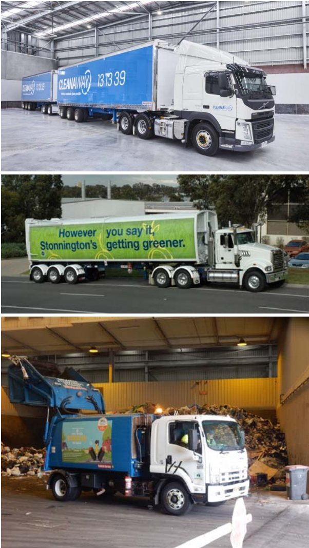
Figure 10.3 : Example transport types – a double and semitrailer bulk linehaul truck, and waste contractor collection vehicle 78
