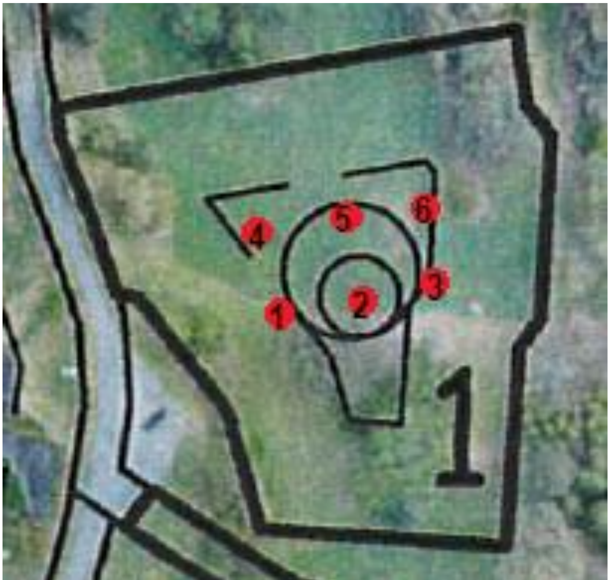
Figure 1. Positions of six repeated soil samples (WL1 R1-6) over intended Lot 1
