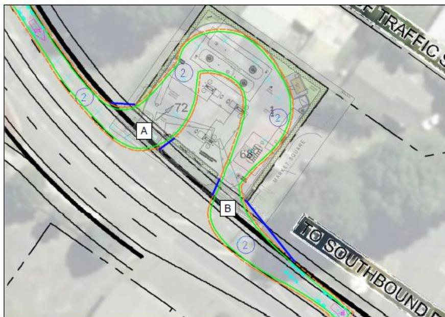
Figure 4: Fuel delivery tanker left turn manoeuvres, from left lane start position (Gray Matter, 18 March 2021)
