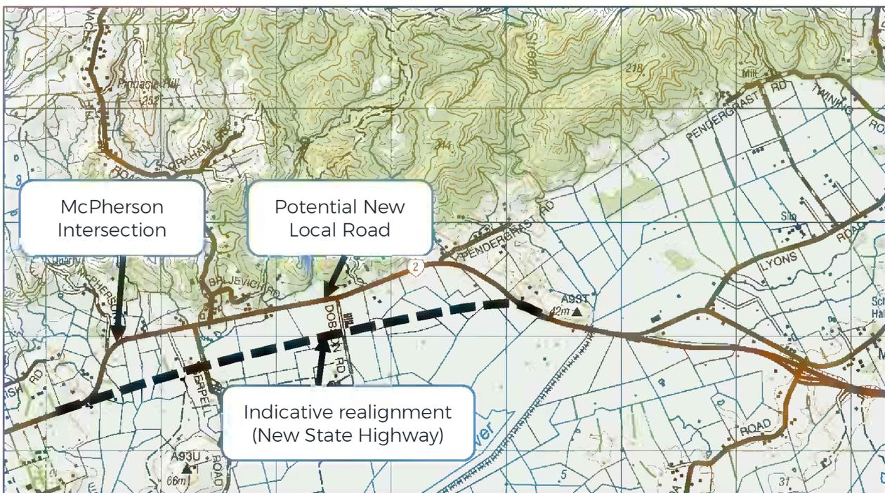
Figure 3: The proposed indicative realignment of State Highway 2 Section A.
