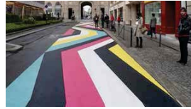
Asphalt surface painting as a visual cue for pedestrian priority.
