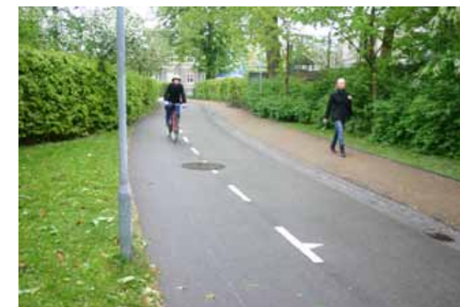
Figure 13 – Surface texture and colour are used on these paths to separate pedestrians from cyclists and to make it clearer as to which paths cyclists and pedestrians are required to use. In one case a spoon drain made of cobble stones provides this separation. In the other case, the separation is achieved by a grassed division.
