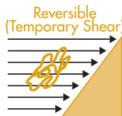
Polymer coil is squashed under temporary shear forces
