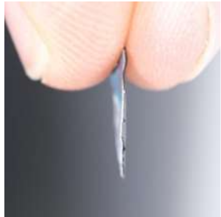
The thickness of the Opal in an Opal triplet can be as little as 0.18mm
