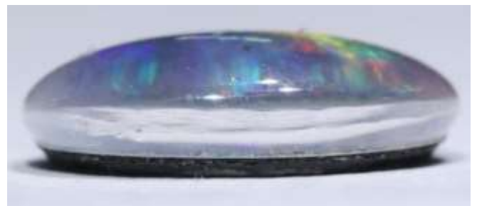
Opal triplet side view - 3 layers -
